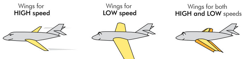
Fig. PF 6.1 Wing design optimisation
