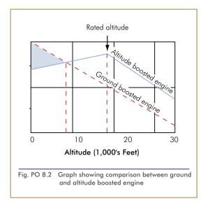
increased by the use of the supercharger, but the power decreases as the aircraft gains altitude, *see fig. PO 8.2.* There are a number of ways that sea level power can be maintained at a specified altitude using superchargers.
