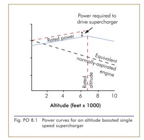
Power will be increased if the manifold pressure is increased, since more air and hence more fuel can be burned per unit time. The power increases because more chemical energy is released per time unit. An increased manifold pressure can be obtained with turbochargers or superchargers. These units are called power augmentation devices. A supercharger is an internal centrifugal compressor mechanically driven from the engine crankshaft, usually through a gear train.
