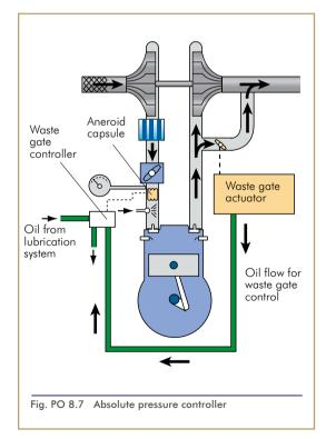
As the throttle is opened towards full power (rated), the turbocharger increases its output until the compressor discharge pressure rises to its maximum permissible value. At that pressure, the aneroid capsule opens the variable orifice bleed valve and oil is bled away from below or to the left of the actuator piston, and spring pressure prevents any further closing of the waste gate. Turbine/compressor RPM and output will be stabilised.
