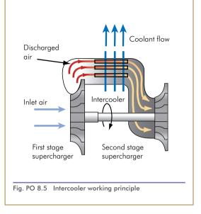
The intercooler cools the compressor outlet air. This also increases the density without reducing the pressure. The intercooler is a heat exchanger. It consists of many tubes in parallel. The hot compressor air flows through the tubes, while ambient air passes over the outside surface of the tubes. The ambient air absorbs heat from the hot air in the tubes and the compressor air gets cooled to a suitable temperature.
