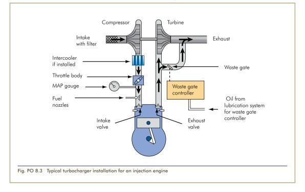
turbine and compressor speed. At sea level rated power can be maintained up to a certain altitude. Maximum altitude at which rated power can be achieved is called the critical altitude, *see fig. PO 8.4.*
