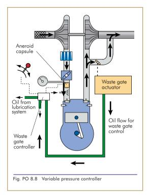
Operation of the throttle to select a specific manifold pressure is matched with a suitable waste gate setting. The operation of the waste gate is as before. With the variable pressure controller the discharge pressure is maintained at 1-2 in Hg above manifold pressure. This relatively low differential pressure reduces the load on the turbocharger and the throttle valve.
