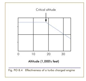
It is usual for turbocharged engines to be ground boosted. There is a critical altitude for every power setting. At the critical altitudes the waste gate is fully closed and maximum turbocharging occurs.
