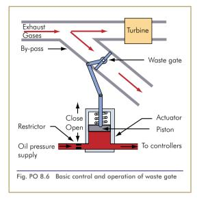
pressure in the actuator causing the waste gate to go more open. A greater amount of the exhaust gases then bypasses the turbine, causing the compressor to deliver less air.
