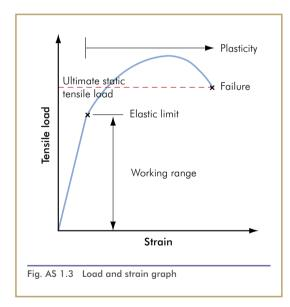
Aircraft are designed so that the different structural members will not be stressed beyond their elastic limits (sometimes termed their yield point) as long as they are operated within their designated limits. Such limits are a main feature to consider in the preparation of Flight and Gust envelopes for particular aircraft types.
