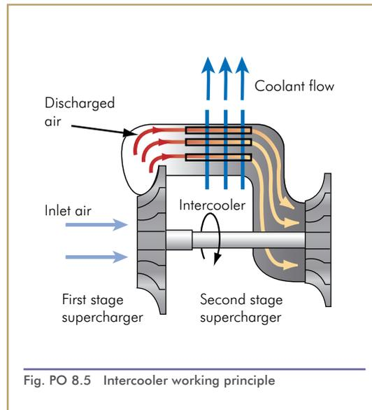
The intercooler cools the compressor outlet air. This also increases the density without reducing the pressure. The intercooler is a heat exchanger. It consists of many tubes in parallel. The hot compressor air flows through the tubes, while ambient air passes over the outside surface of the tubes. The ambient air absorbs heat from the hot air in the tubes and the compressor air gets cooled to a suitable temperature.
