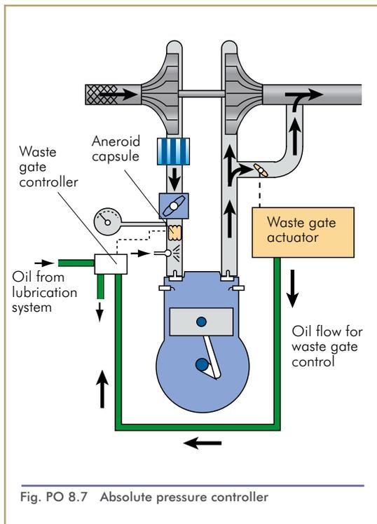
Fig. PO 8.7 Absolute pressure controller
