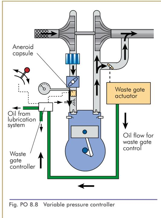
Operation of the throttle to select a specific manifold pressure is matched with a suitable waste gate setting. The operation of the waste gate is as before. With the variable pressure controller the discharge pressure is maintained at 1-2 in Hg above manifold pressure. This relatively low differential pressure reduces the load on the turbocharger and the throttle valve.
