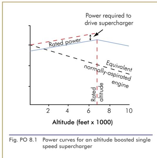
Fig. PO 8.1 Power curves for an altitude boosted single speed supercharger
