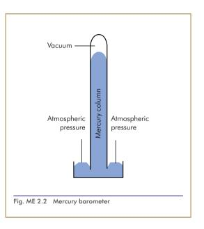
Atmospheric pressure forces mercury to rise in an evacuated glass tube.
