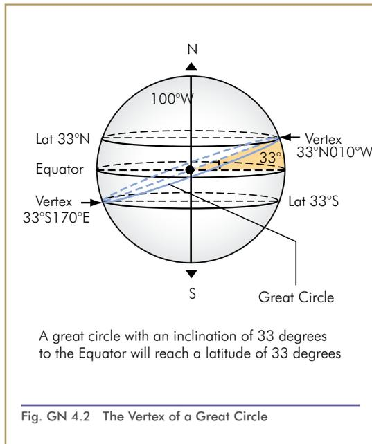
inclination of  $33^{\circ}$  as it crosses the Equator, which is an angle of  $57^{\circ}$  to the meridian. From this perspective it is easy to see that the Great Circle, on its path northeasterly from the Equator, will reach higher latitudes. The highest latitude reached will be the same as the inclination to the Equator i.e.  $33^{\circ}00'N$ .
