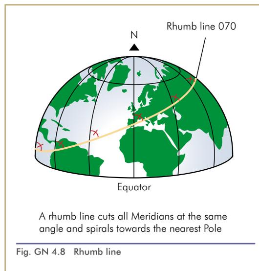
It can mathematically be proven that such a spiral never actually reaches the pole. However this is of no practical interest in air navigation, and we will discuss the Rhumb Line as if it is running as a spiral from Pole to Pole.
