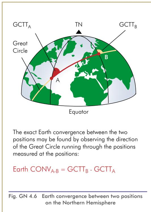
directions, it does illustrate that the true direction of the Great Circle, as it passes through A, (labelled  $GCTT_A$  on the sketch), is of a lower value than the true direction of the Great Circle as it passes B.
