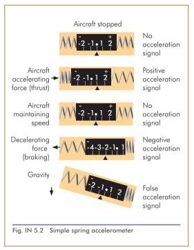
The accelerometer cannot calculate velocity or distance itself, it quite simply registers the spring displacement, which is directly proportional to the accelerating or decelerating forces. Velocity and distance are computed from sensed acceleration by the application of basic mathematical formulas of integration.
