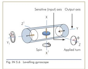
The gimbal or gyro precession around the output axis is thus proportional to the rate of rotation producing it. The pickoff measures this precession and passes a voltage proportional to the precession to the relevant gimbal torquer, which drives the gimbals to keep the platform level and aligned. In addition each gyroscope has a gyro torquer which is used to apply forces to the output axis to correct for apparent drift and topple.
