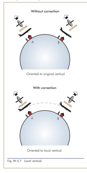
and this alignment must be maintained if the correct accelerations are to be measured. Moreover, the sensitive axes must be kept perpendicular to the gravity vertical, otherwise, the accelerometers sense part of the gravity acceleration *(fig. IN 5.7)*. The reference frame defined by these directions, i.e. local North, local East, and local Vertical, is called the Local Vertical Reference Frame. Other reference frames can be used, but the local vertical is the fundamental mechanisation used.
