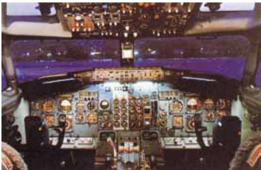
Fig. IN 1.1 Cockpit B737-100
